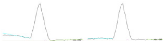
Figure 4: Data before and after drift fixing procedure. The best fit lines are shown in blue and green.
