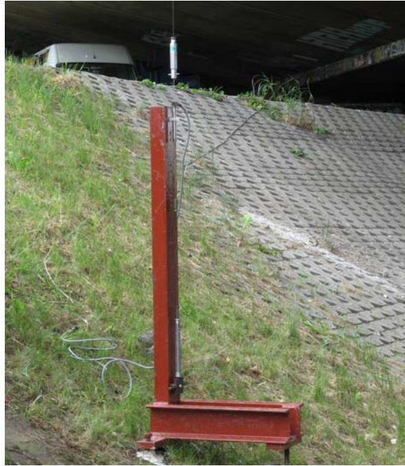
Fig. 134 - View of the device for measuring relative deflection KSM-R sensor tracks WA50 captured in section R91
