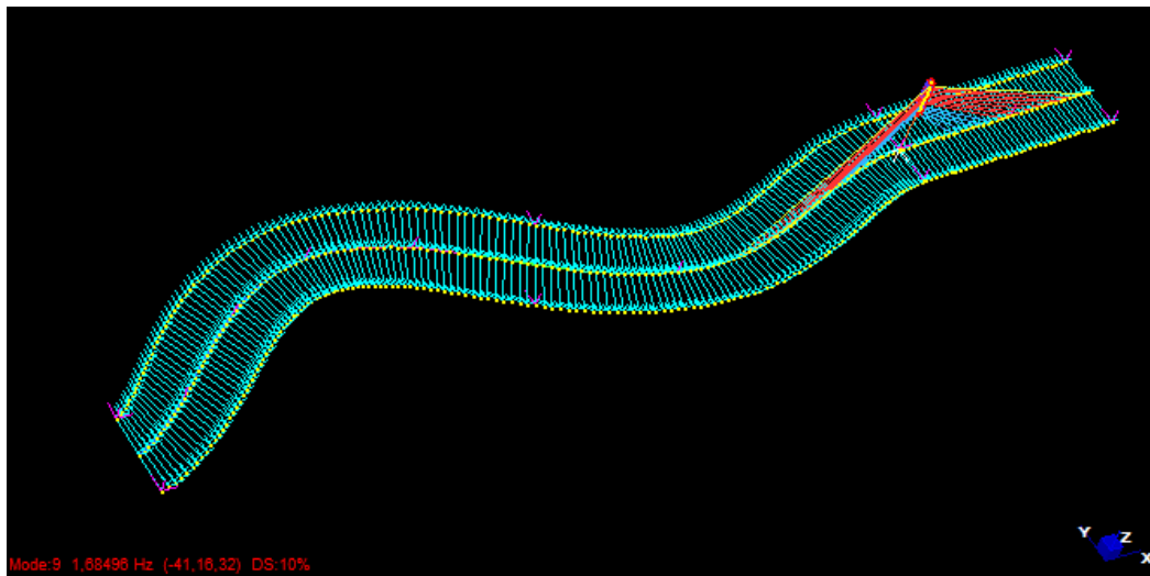
Fig. 105 - Fifth natural mode (beams model with masses)
