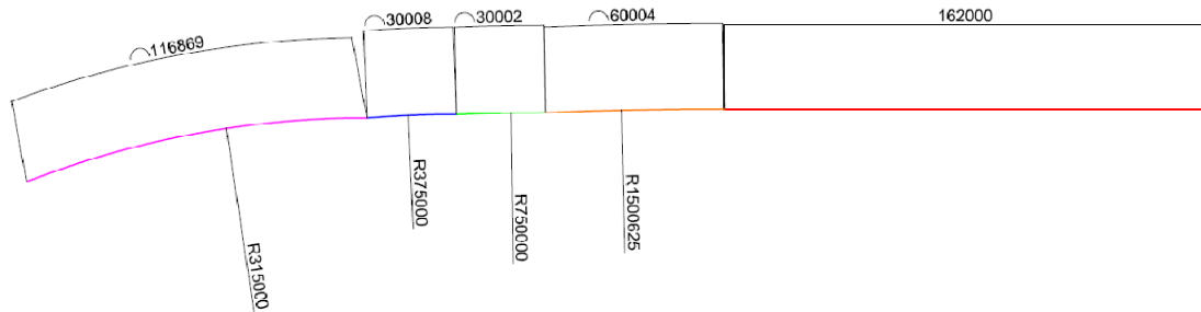
Fig. 30 - Track of the bridge (mm)
