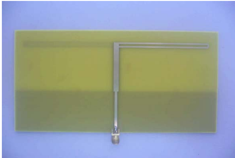
Figure 3.13: Front side photograph of the double sided planar folded dipole
