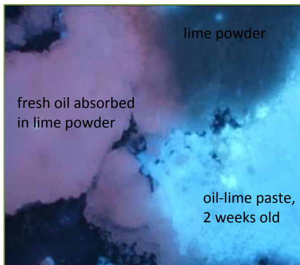
Figure 34: Fluorescence of oil-lime paste compared to lime without oil and lime with applied oil drop
