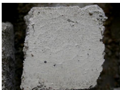
Figure 78: Formation of crack due to freeze on the surface of a specimen (code C1O 1 )
