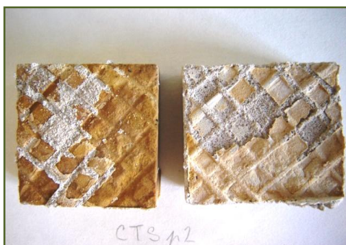
Figure 3: Decomposition of mortar-stone composite sample: Surface layer of cretaceous marly chert (left) was detached by cement-hydraulic lime mortar (1:1) (right) after three sodium sulfate crystallization cycles (78)
