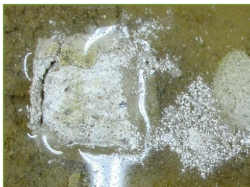
Figure 75: Specimens of hydrated lime and brick dust mortars in sodium sulphate solution - specimens are hydrophobic, they lose surface powder layer
