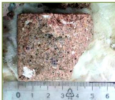
Figure 71: Specimen after 6 hours of full immersion into a salt solution - solution penetration only into depth of approx. 3 mm
