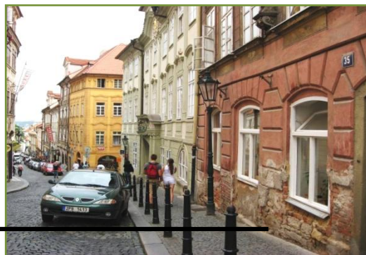
Figure 7: Example of masonry damaged due to the crystallization of salt on a frequent street in Prague, Czech Republic, where NaCl is used as a de-icing agent in winter
