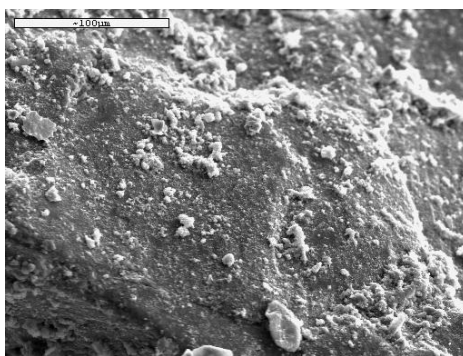
Figure 69: Pozzolanic mortar with 1% oil addition (code PO 1 ) after twenty NaCl crystallization cycles performed (SEM)
